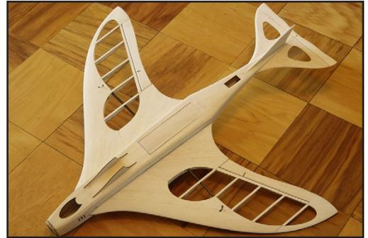
41. Check Center of Gravity against the plans and ensure you are within 1/8". Position the battery to adjust the C/G, and mark the battery's position. Use velcro to hold the battery in place.
