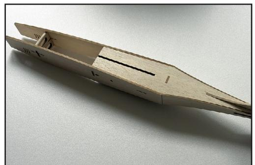
there is good contact with body. Use thick CA or epoxy for a strong joint.
