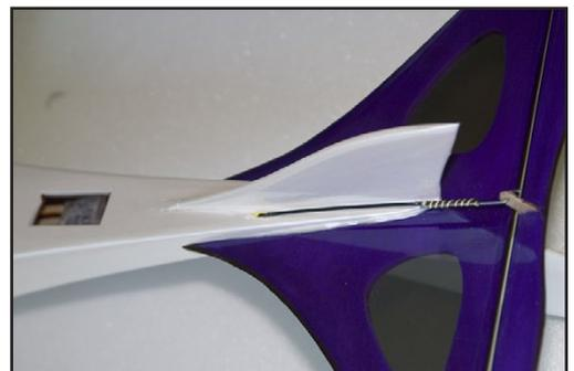
39. The wing can be left unglued if you wish it to remain removable, however, for increased strength the wings should be glued to the body. Use the supplied carbon tube to join the main carbon wing spars inside the body. Use rubber bands to hold wing in place while glue dries.
