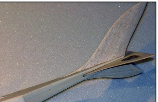
30. Trim excess sheeting. Use a straight edge and a sharp X-acto knife to trim at the root rib. Check fit with body before trimming.
