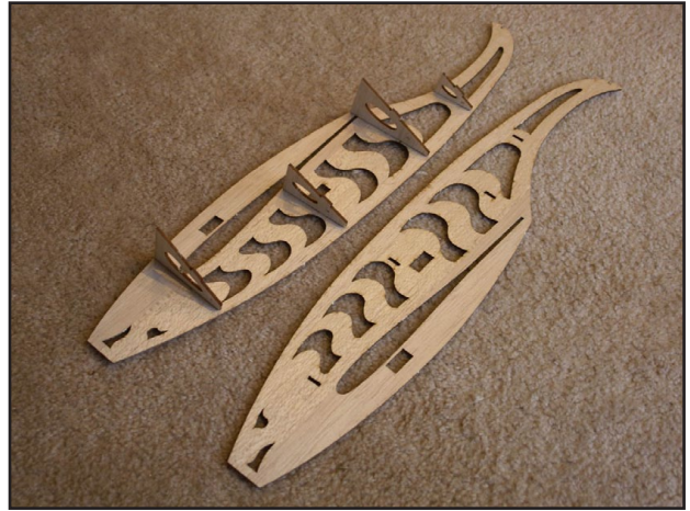
Assemble and glue inner body braces A, B, C, D to one side of body, then glue two body halves together with vertical tail fin sandwiched and glued in-between body halves.
