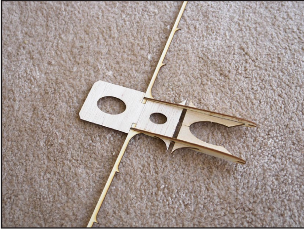
Assemble and glue the inner wing pieces and trailing edge pieces as shown above.
